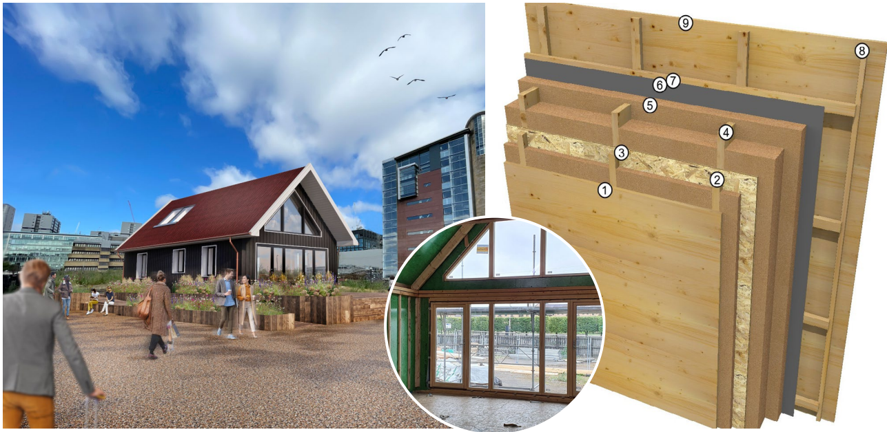
The COP26 House wall build up features 1) 22 mm timber boarding internally; 2) on battens with 40 mm Steicoflex insulation; 3) on 12 mm Medite Propassiv boards; 4) on timber studs with 140 mm Steicoflex insulation; 5) on 80 mm Steico Special Dry boards; 6) on Steico UDB breather membrane; 7) on 30 mm battens 8) and 30 mm counter battens; 9) on timber cladding.
